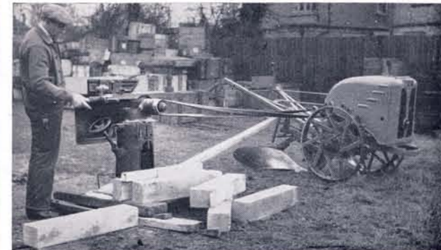
Power Take-off driving Saw
